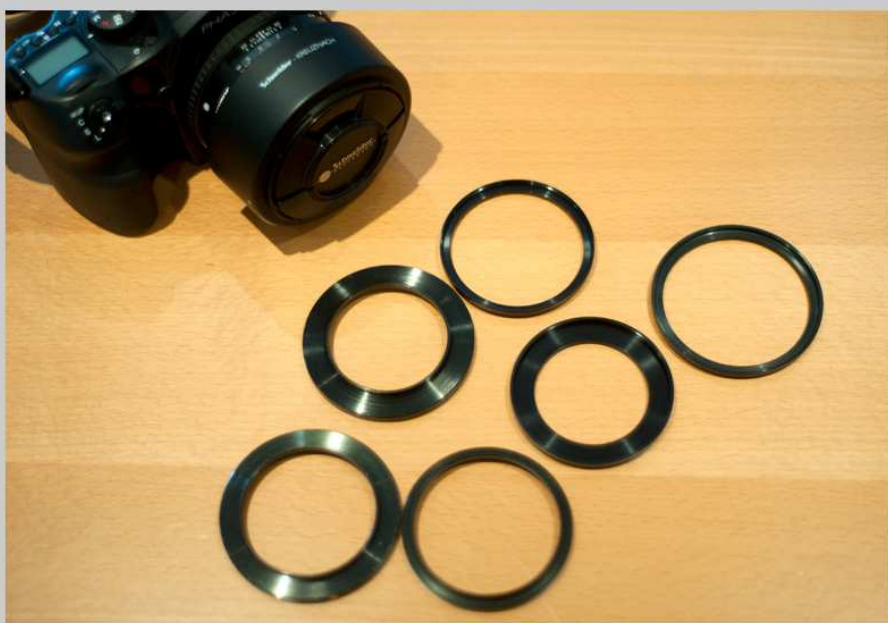
Step up rings let you attach a single ND filter to lenses with various diameters
