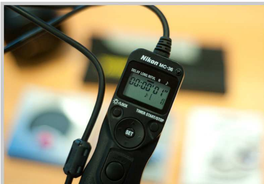
Nikon cable release with built in timer for long exposures.
